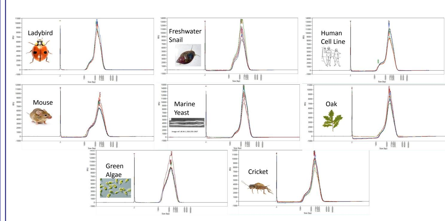
The Oak, Mouse and Green Algae pools were selected for sequencing. To optimise the sequencing results a size selection was performed using a sage science PippinHT instrument. Traces from the Agilent Femto Pulse showing the size distribution of the pools after size selection are shown below.
