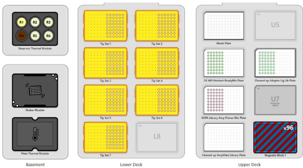
Figure 4. Starting deck layout for Protocol 4 of 4: 4.1 - 4.3 Library Amplification and Purification. Example shown is for 6 columns of samples.
