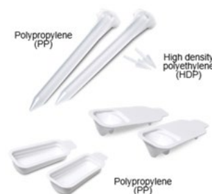
Figure 3. (a) Reservoir and tip type comparison. *SPT Labtech firefly/dragonfly reservoir (1 g), SPT Labtech firefly/dragonfly syringe (4 g). †LP SBS 96-well diamond bottom reservoir weight (23.3 g) based on Axygen (RES-SW96-LP), other SBS reservoir types may differ. §Single tip weight (1.6 g) based non-filter 125 \mu L apricot tips, other tip weights may differ. ‡Tip box not included in weight calculation. (b) SPT Labtech's firefly and dragonfly syringe and reservoirs.
