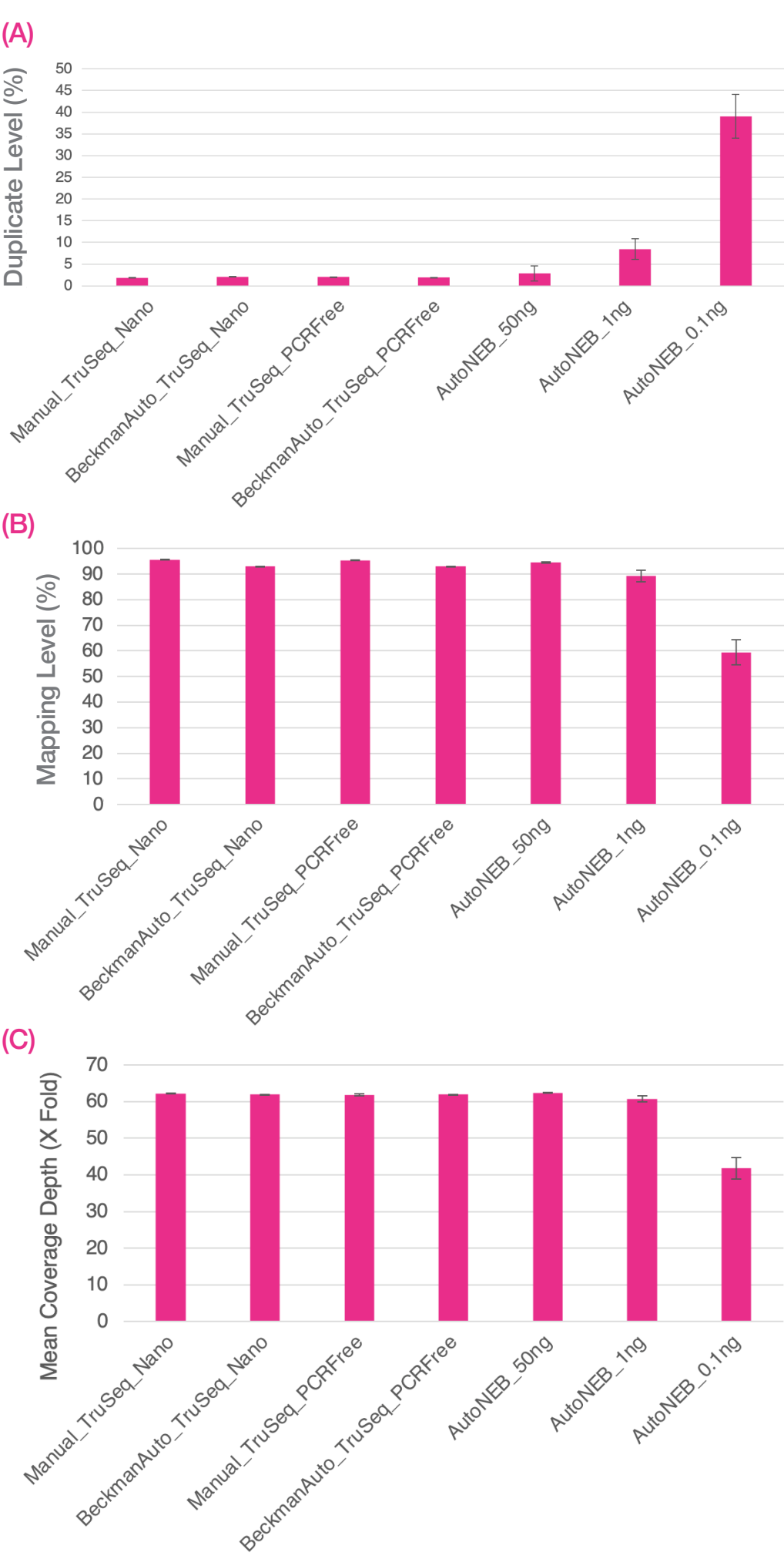
Figure 6. Sequence data were normalized to 1.3M reads per library. Bar charts show averages of A) percentage duplicates, B) percentage mapping, and C) fold coverage (X) of the mock community. Error bars are standard deviation.
